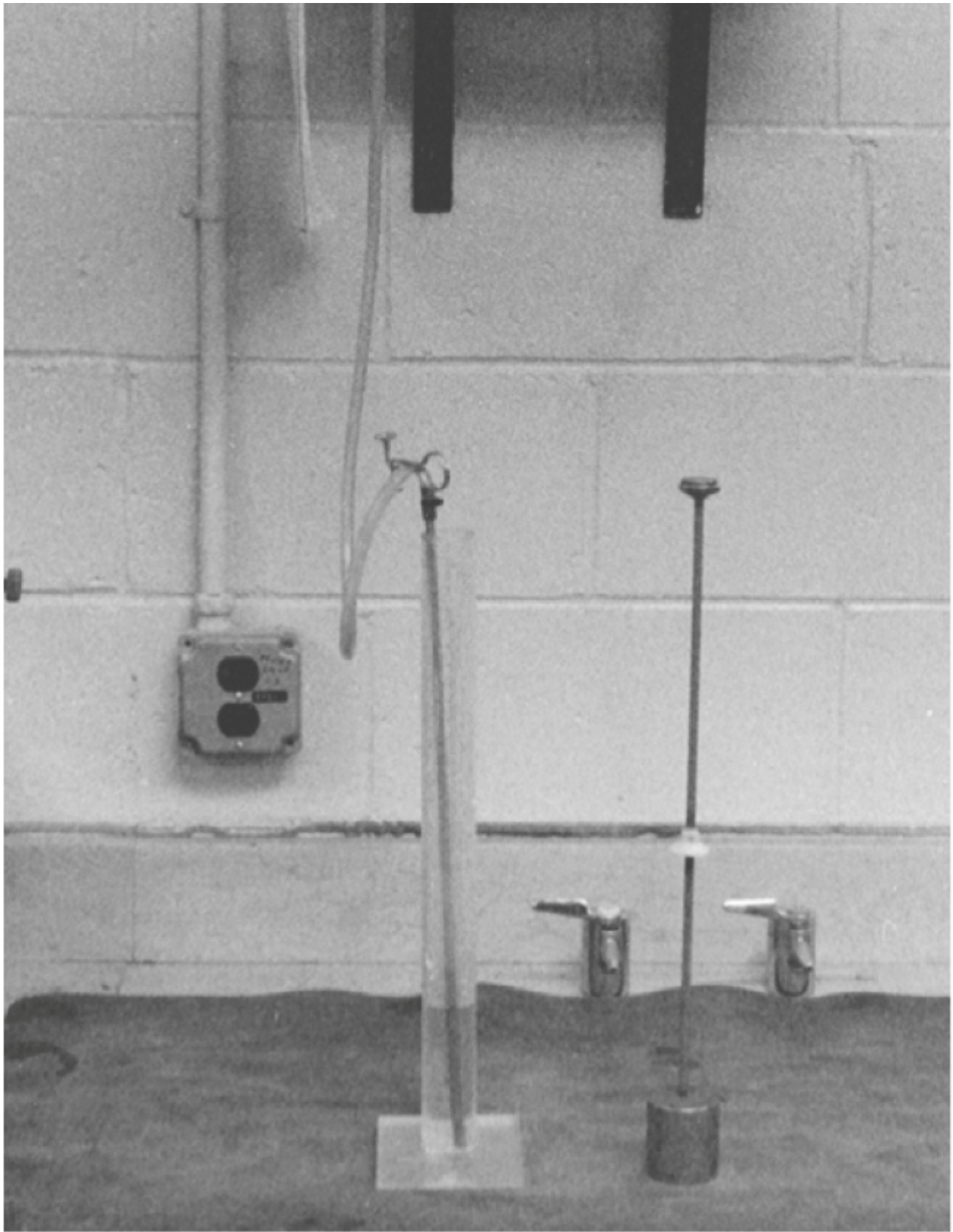
Figure 2 —Graduated Cylinder, Irrigator Tube, Weighted Foot Assembly, and Siphon
