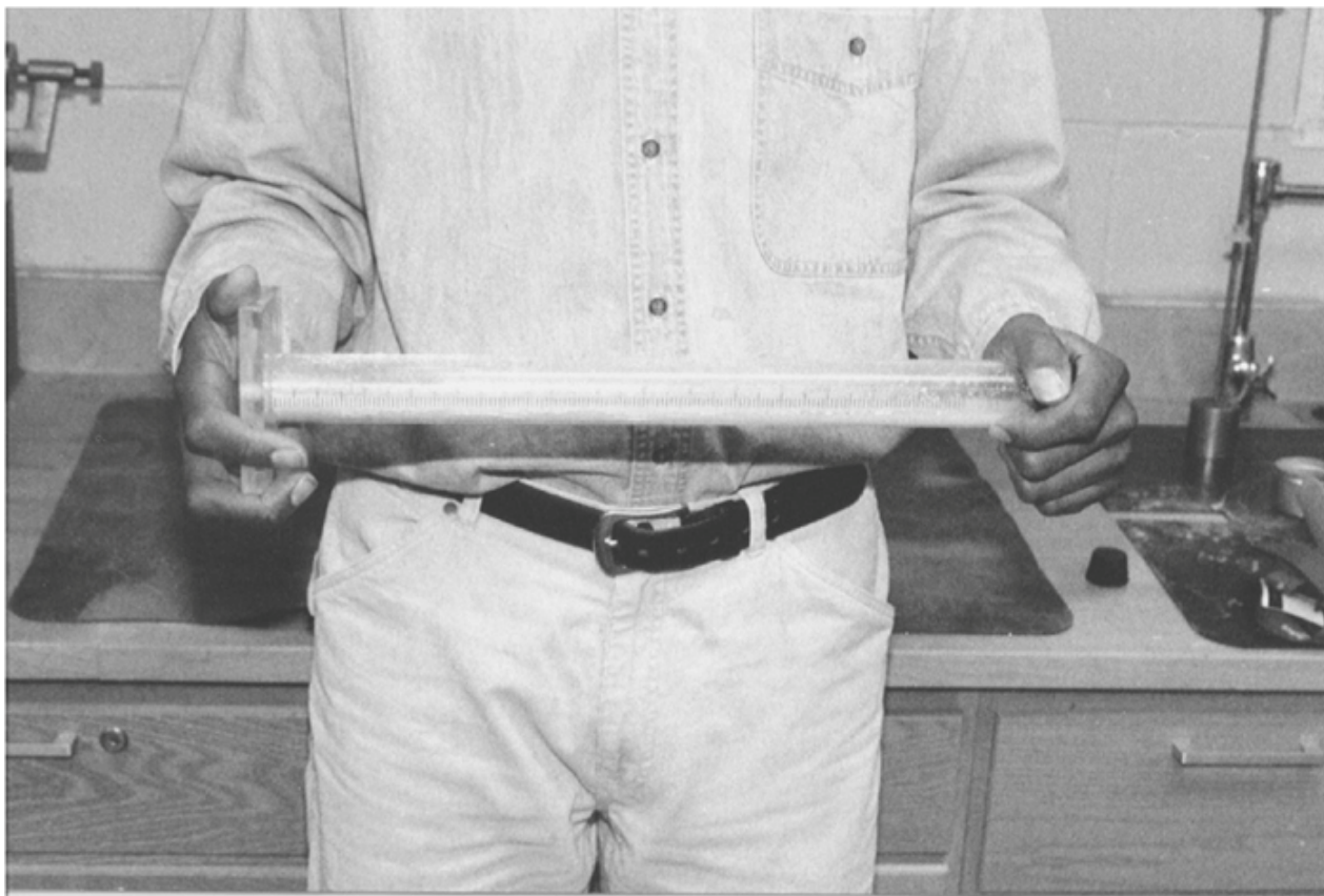
Figure 4 —Using Hand Method of Shaking
