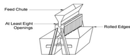
Riffle Sample Splitter (a) Large Sample Splitter for Coarse Aggregate
